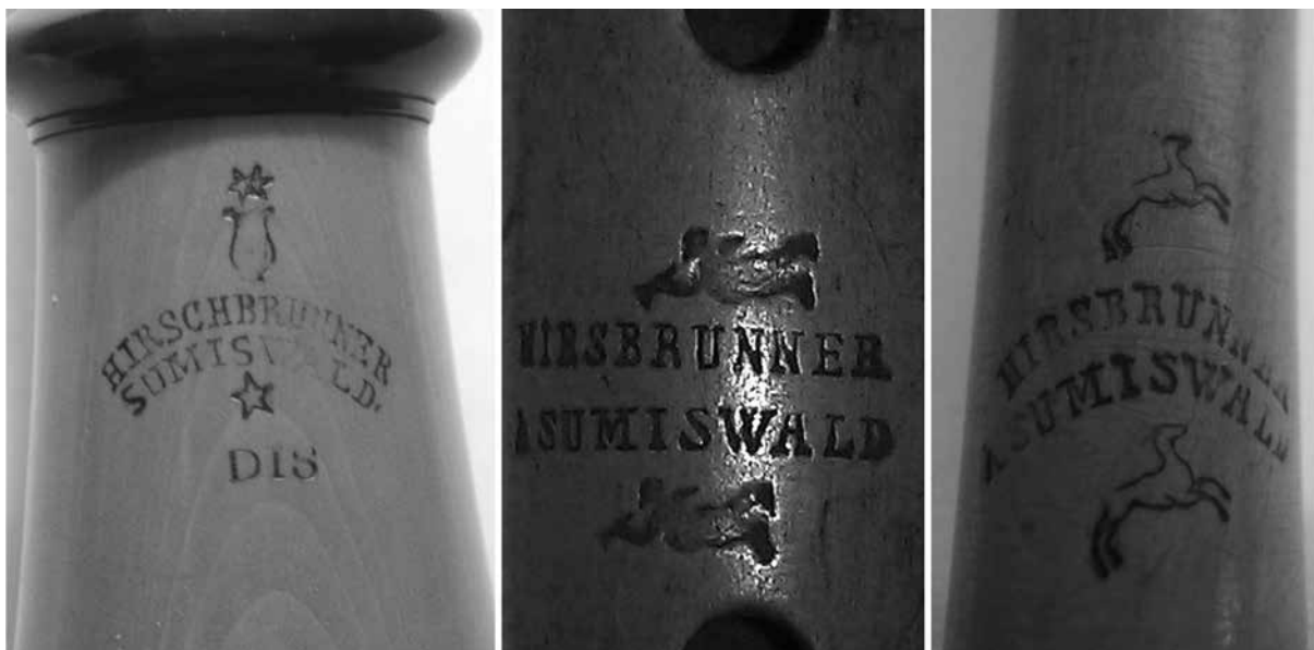
Figures 3, 4 and 5. The three different inscription styles found on Hirsbrunner woodwind instruments: curved stamp 'HIRSCHBRUNNER / SUMISWALD' with lyre and stars; straight stamp 'HIRSBRUNNER / A SUMISWALD' with trumpeting angels or suns; and curved stamp 'HIRSBRUNNER / A SUMISWALD' with deer.
