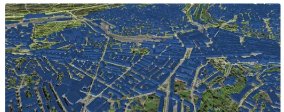
Rendering of the Buildings3D dataset and the street network from the topological landscape model on top of the terrain.
