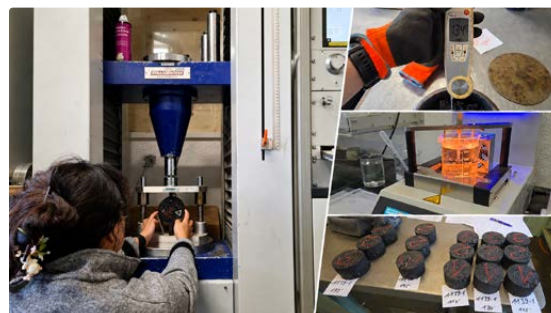
Laboratory programme: specimen preparation, binder recovery and performance testing
