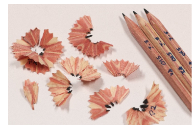
Evaluation of pencils produced with local wood impregnated with solution of paraffin and dyes.
