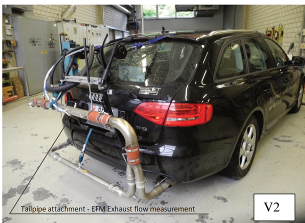
Fig. 3. Tested vehicles (FFV) equipped with PEMS
