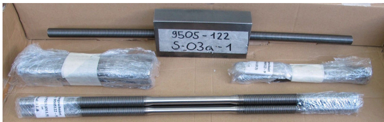
Figure 2: Steel specimens; connection with internal thread (top) and machined threaded rods (bottom)
