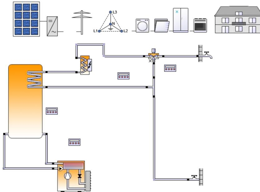
Figure 4: Simulation scheme in the software Polysun.
