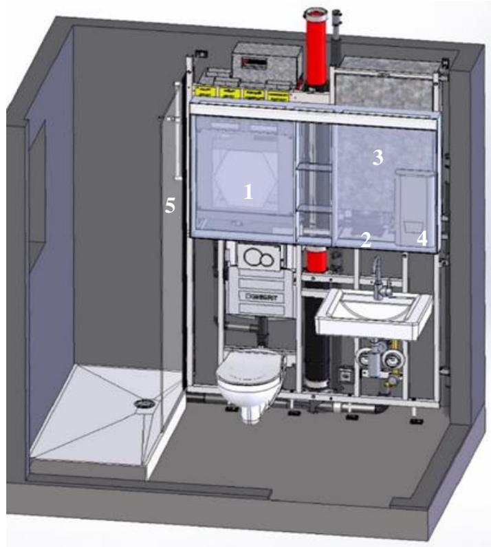
Figure 1: DHW system in the bathroom prewall.
