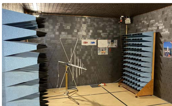
OFCOM — Semi-Anechoic Chamber used for EMC measurement
