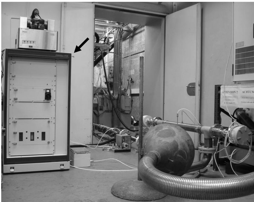
Figure 4: FTIR (arrow) and sampling line in the IC- engines laboratory in Biel
