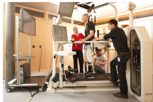
Fig. 2: Lokomat exoskeleton rehabilitation robot.
