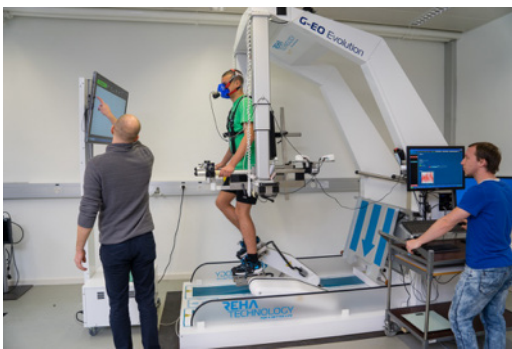
Fig. 1: G-EO System end-effector rehabilitation robot
