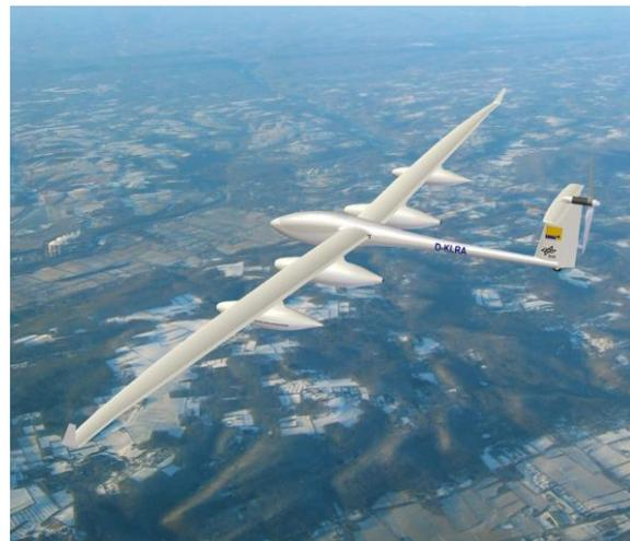
Figure 12: Model of the Antares DLR-H3 which should make 6’000 km range with the fuel cell
