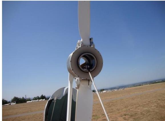
Figure 10: View into the DC - motor of the Antares 20E
