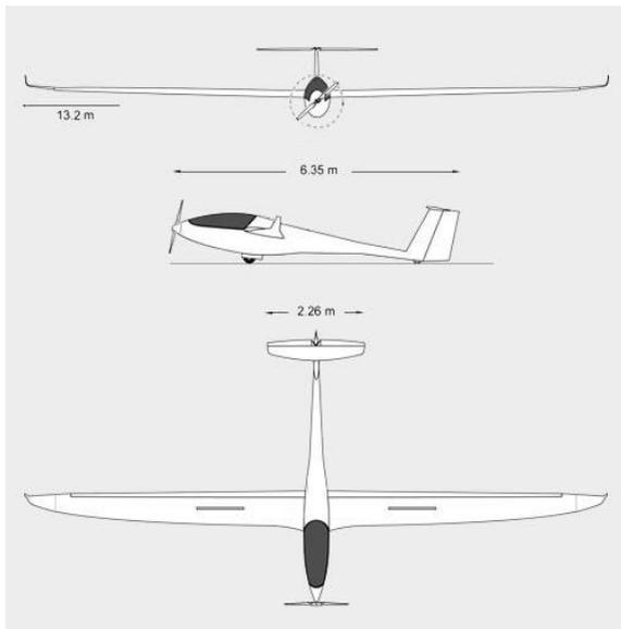
Figure 13: The Silent 2 Electro glider from Alisport Srl (Italy)
