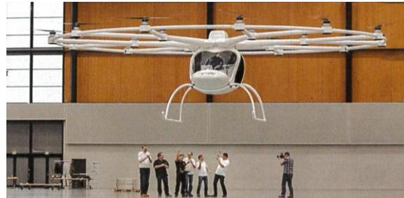
Figure 19: German project Volocopter a 2-seated multicopter with E-drive
