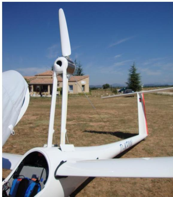
Figure 11: Small propeller beam with retractable motor and propeller system of the Antares 20E
