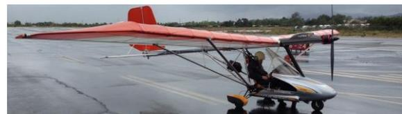
Figure 17: E-spider from Yuntec and marketed by GreenWind International (USA)
