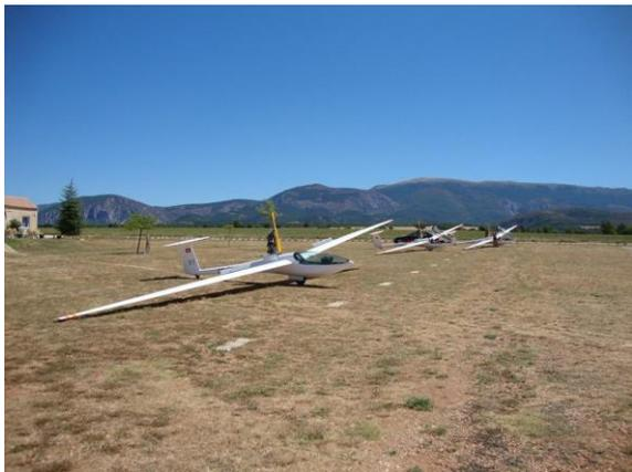
Figure 3: Three DG 400 with retractable 2-stroke motor produced since 1982
