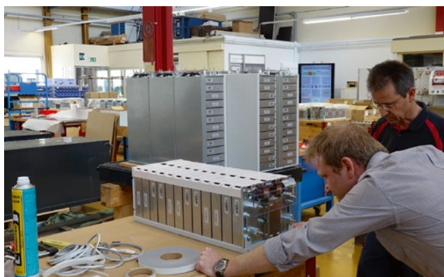
FIGURE 2 Assembly of the battery pack (total 16 stacks per battery) (© Lithium Storage)
