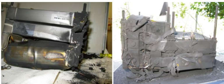
FIGURE 9 Temperatures during the spread test, cells after the spread test (© Empa Dübendorf)
