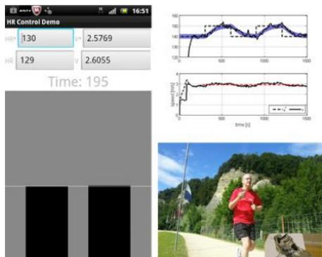
This work has shown that, even during outdoor running, very precise tracking of HR profiles can be achieved, with root-mean-square tracking errors of less than 2 beats per minute.
