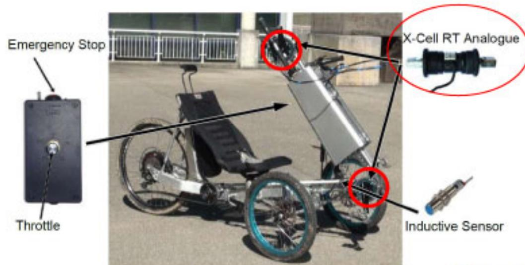
Figure 28: Wireless FES cycling sensor setup. Emergency stop, throttle, torque sensor, encoder and inductive proximity sensor mounted on the trike
