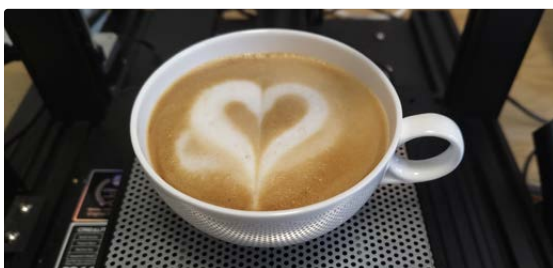
Figure 1: A heart pattern produced by the system using real milk foam, defined entirely as a software tool-path
