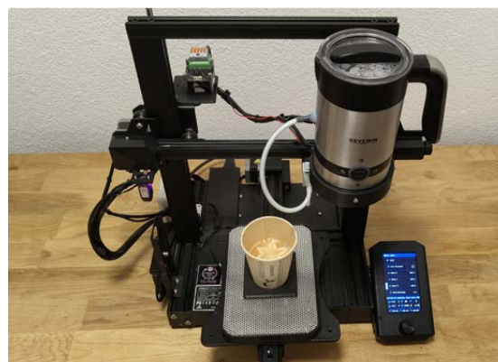
Figure 2: The automated latte-art maker, a three-axis gantry built using a modified 3D printer, with a foam-dispensing valve and a stylus tool positioned over the cup
