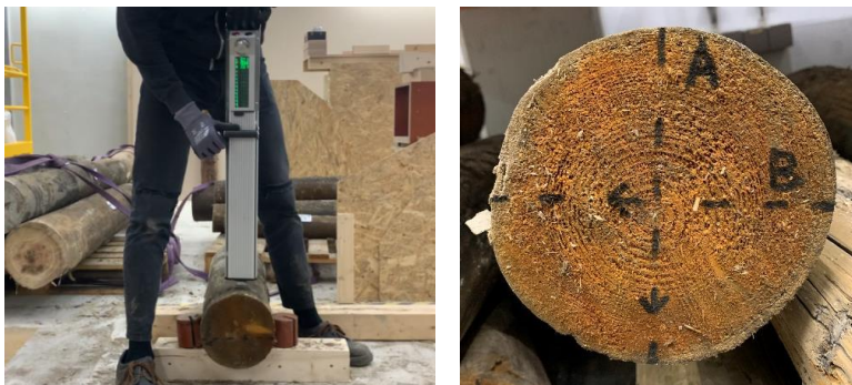
Figure 5: Micro-drilling measurements performed on a pile segment before the compression test.
