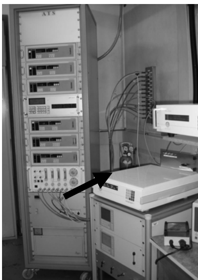
Figure 3: CLD analyzer (arrow) and sampling line (circle) at the test stand
