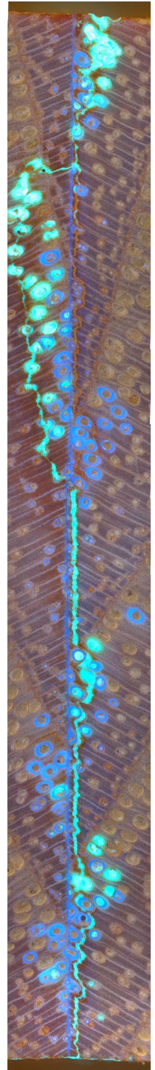
Fracture analysis of Ash wood glued sample; the original glue line is shown in dark blue, the breaking line is shown in green
