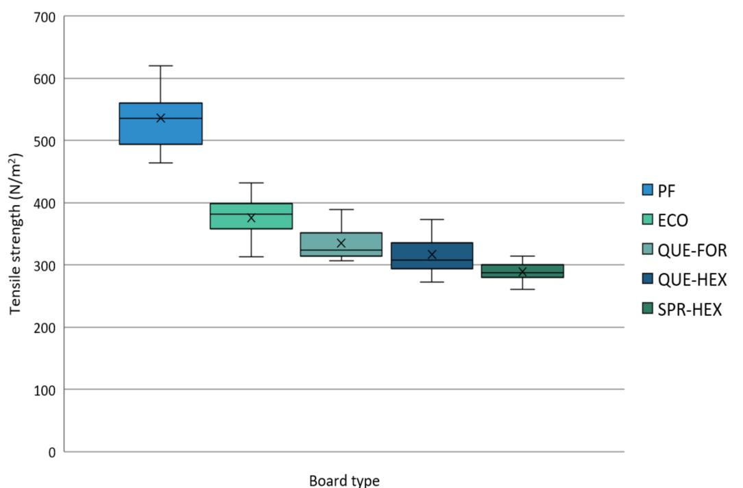
Figure 2. Results from the tensile strength test, n=16, for different adhesive systems
