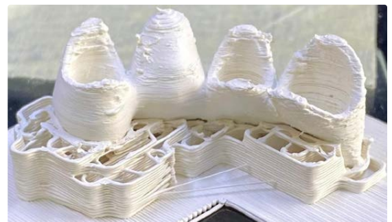
Zirconia-based FDM-manufactured dental crown.
